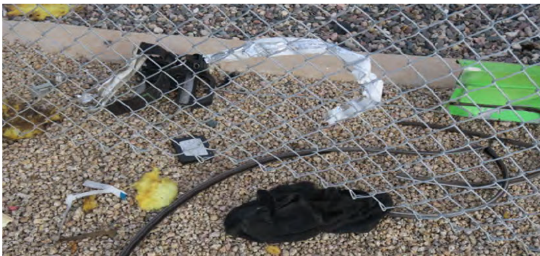
Figure 4.17: Photograph of firefighter equipment removed by the fence during the deflagration [6].
